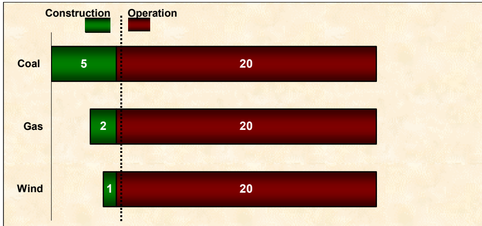
Figure 2. Construction lead time for coal, gas, and wind plants
