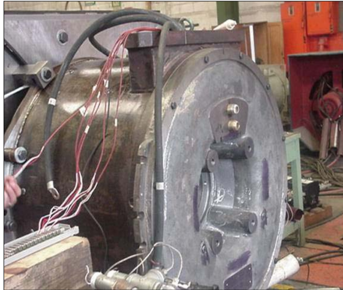
Figure 4. One of four permanent-magnet generators for the DGD4 Quantum Drive
