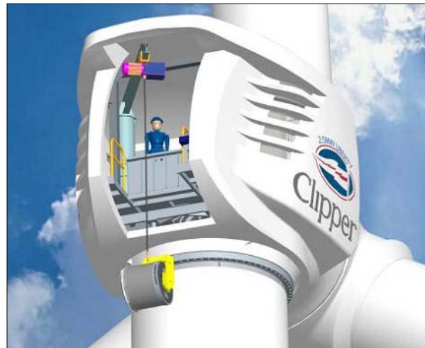
Figure 9. Rear door and cooling vents in the nacelle
