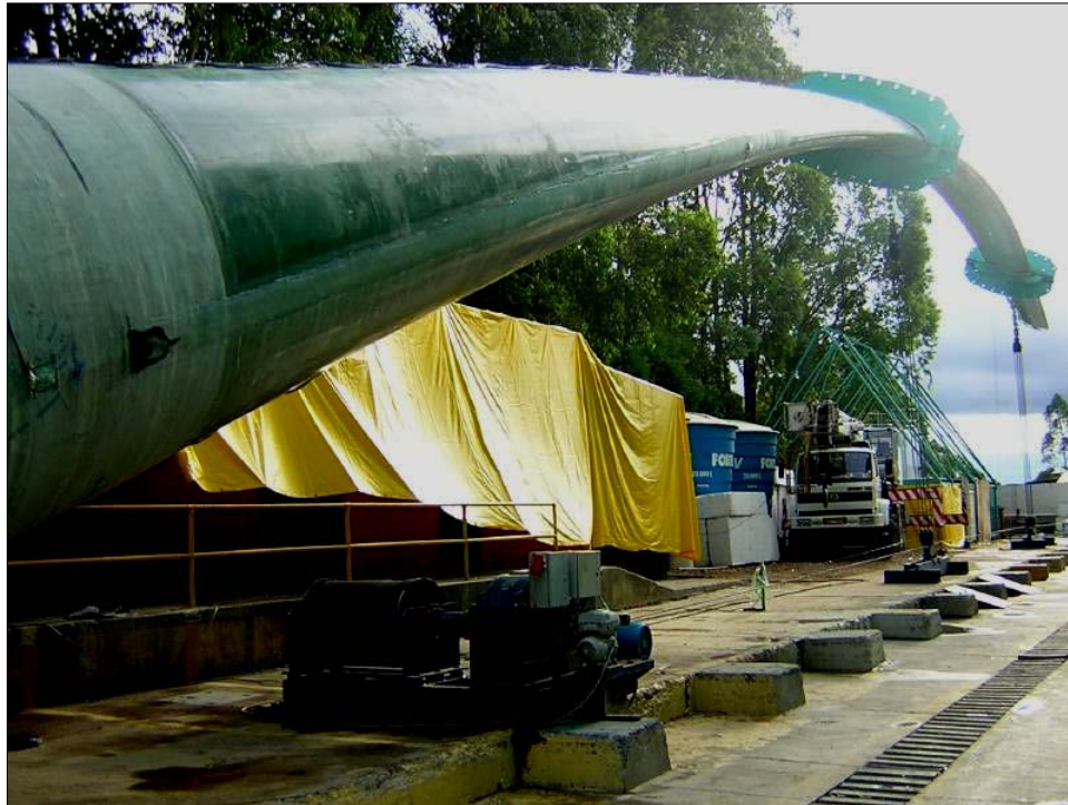
Figure 6. C93 truncated prototype blade undergoing static loads test on November 17, 2004
