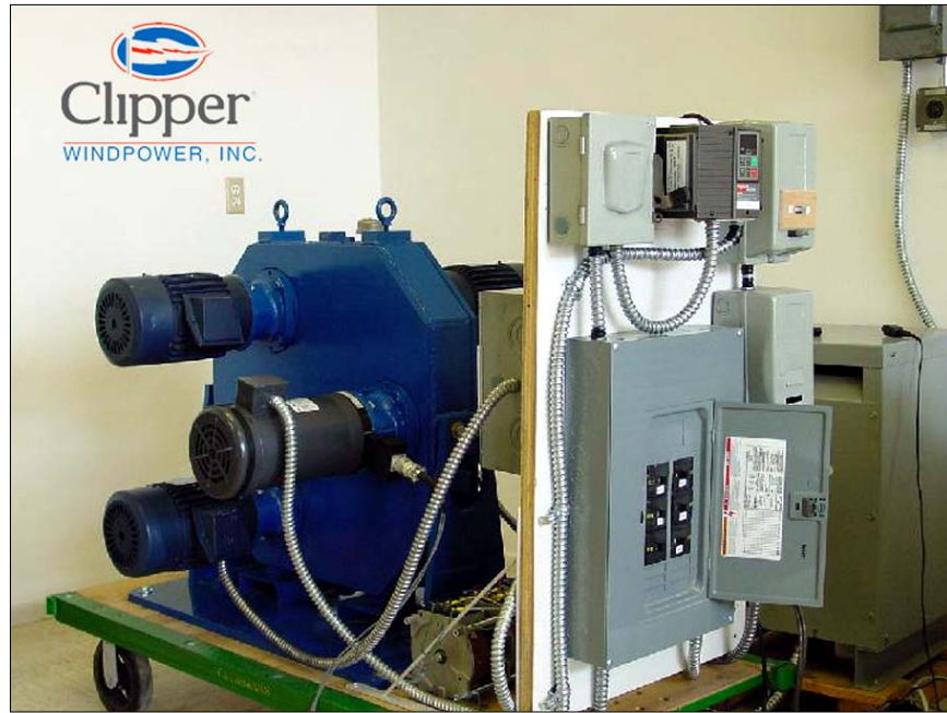
Figure 1. Lab-scale DGD (this test equipment was used in the investigation and development of controls specific to multiple generators)
