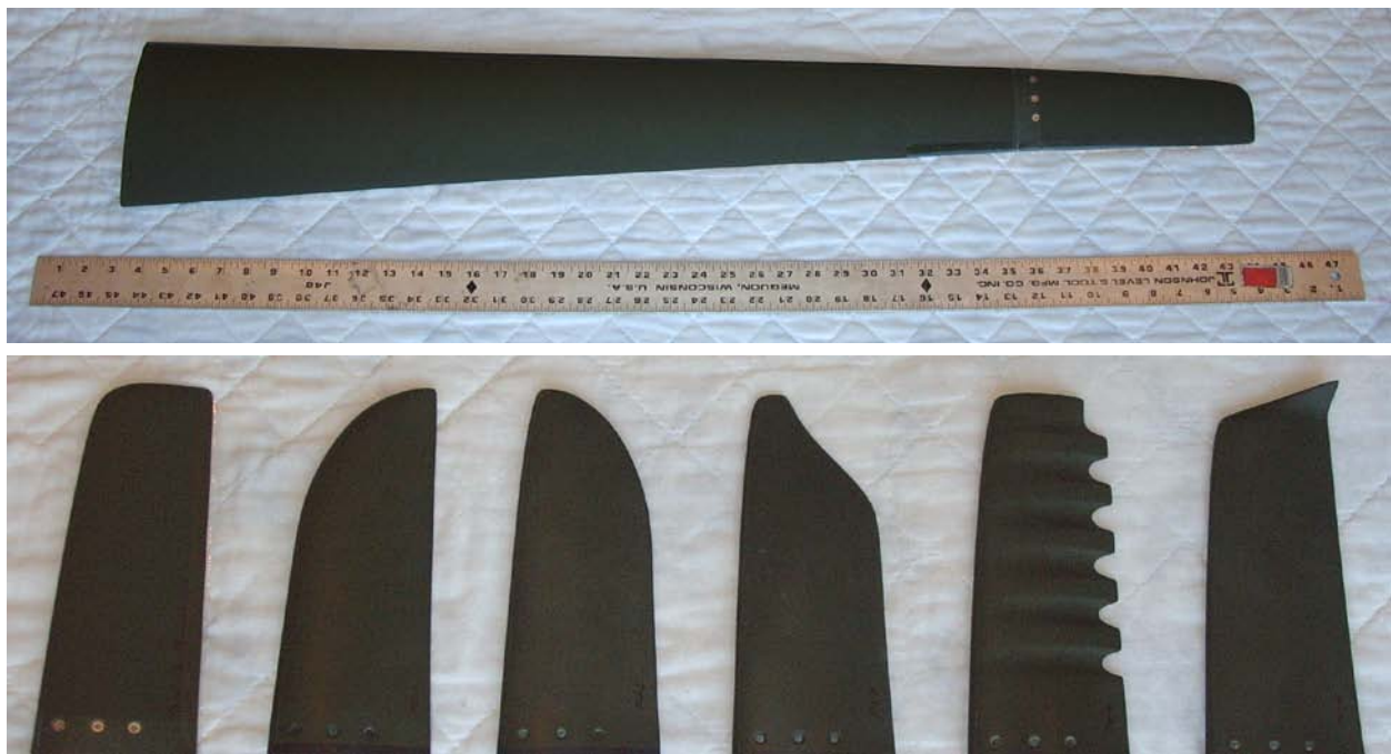
Figure 5. Wind turbine blade segment used for the test model (top photo) and the removable blade tips (bottom photo) – from left to right –Storm baseline blade tip and removable tips PM-1 (leading edge sweep), PM-2 (trailing edge sweep), PM-3 (ogee shape), PM-4 (scalloped trailing edge) and PM-5 (winglet)
