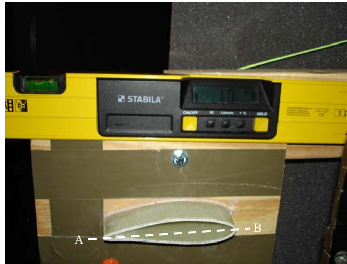
Figure 4a. Angle of attack was measured with an electronic level.
