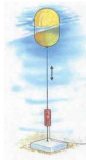
Figure 1 – Point Absorber Schematic.
