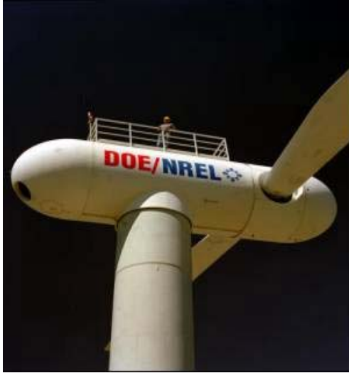
Figure 1. The controls advanced research turbine (CART).
