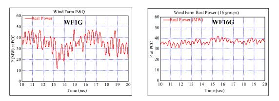
Fig. 3. Real power output of a wind farm in a WF1G and in a WF16G.
