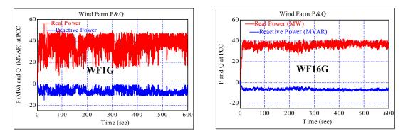
Fig.4. Real power output of a wind farm in a WF1G and a WF16G.
