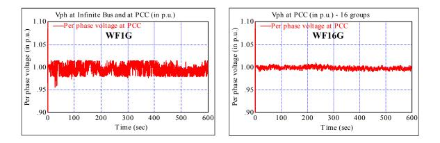
Fig. 5. Comparison of voltage variation at PCC for the wind farm models WF1G and WF116G.
