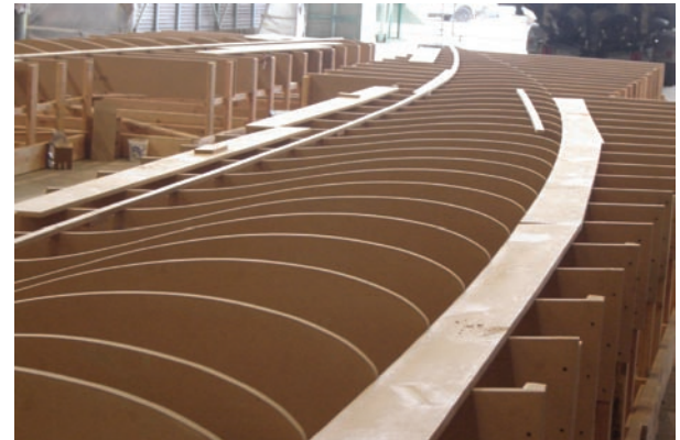
The initial mold fabrication for Knight and Carver's sweep twist blade.
