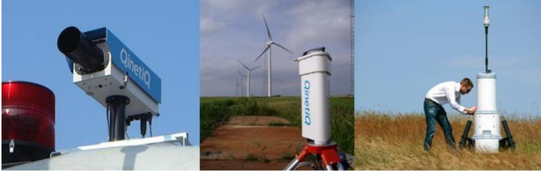
Figure 3. Stages of evolution of the ZephIR lidar. Figure 3a shows the lidar head mounted on the nacelle of a Nordex N-90 wind turbine. Figure 3b shows prototype ground-based wind profiler at Risø wind energy test site, Høvsøre, Denmark. Figure 3c shows the ZephIR production model deployed in the field
