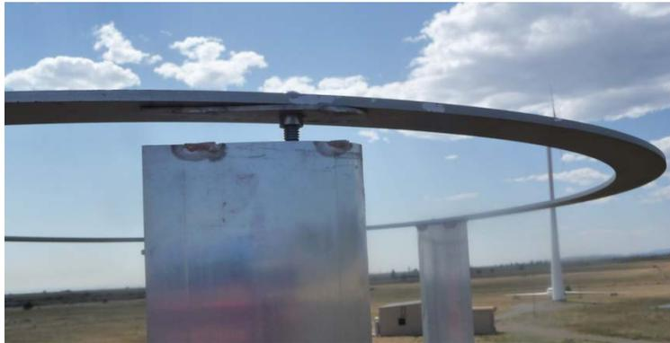
While the leading edge tape was being replaced (due to detachment), a broken weld was found at the top of the turbine and another crack was observed on a different weld. Initially, the welding was done in two spots per airfoil side. The airfoils also slid out of the struts that are supposed to clamp them. This may have caused the broken weld. The turbine was visibly wobbling and was tilted down.
