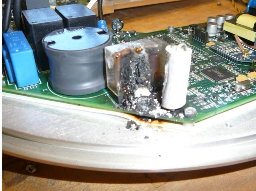
The inverter failure occurred because the set points of the inverter were set to optimize power performance. The increased performance caused the temperature to rise, and over time, caused the inverter to fail. The inverter was replaced. The set points were set for normal production.
