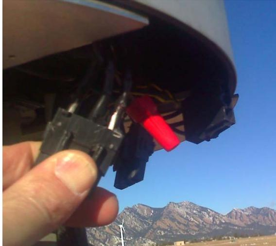
The testing team checked the turbine after it observed possible higher rotational speeds while the turbine was shut off. Measurements that were taken to check for generator continuity were varied when they should have been less than 5 ohms. The team found that two of the three wires from the generator were missing insulation and bare wire was exposed. There was no noticeable difference in resistance when force was applied while the generator was connected or not.
