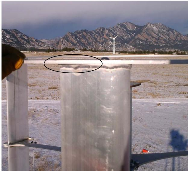
During the noise testing, a clanging sound emanated from the turbine. The testing team found two broken welds at the top of the turbine. The turbine was shut down until further notice. This photo shows one of the broken welds that caused the airfoil to separate from its end plate. However, the airfoil did not completely separate as it did in the previous occurrence.
