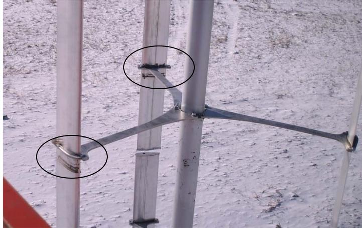
Two out of three airfoils slid down through the struts. In the picture, the black markings show where the airfoils used to be.
