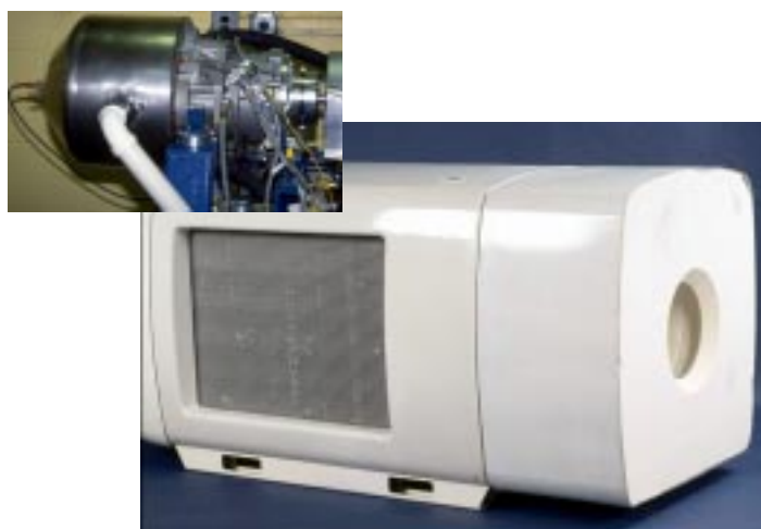
Figure 2. STM power conversion system package comprising the thermal receiver, the Stirling engine, and the generator. Solar energy enters the receiver through the aperture on the right side of the enclosure. The insert shows a gas-fired engine under test.
