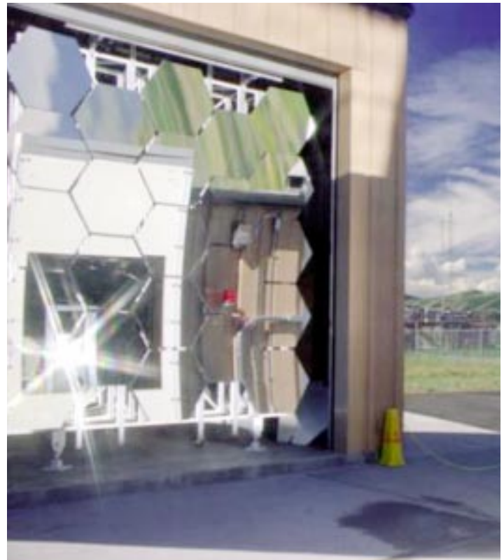
At NREL's High-Flux Solar Furnace, a large flat mirror tracks the sun and reflects solar energy onto 25 individual curved mirrors, collectively known as the primary concentrator.
